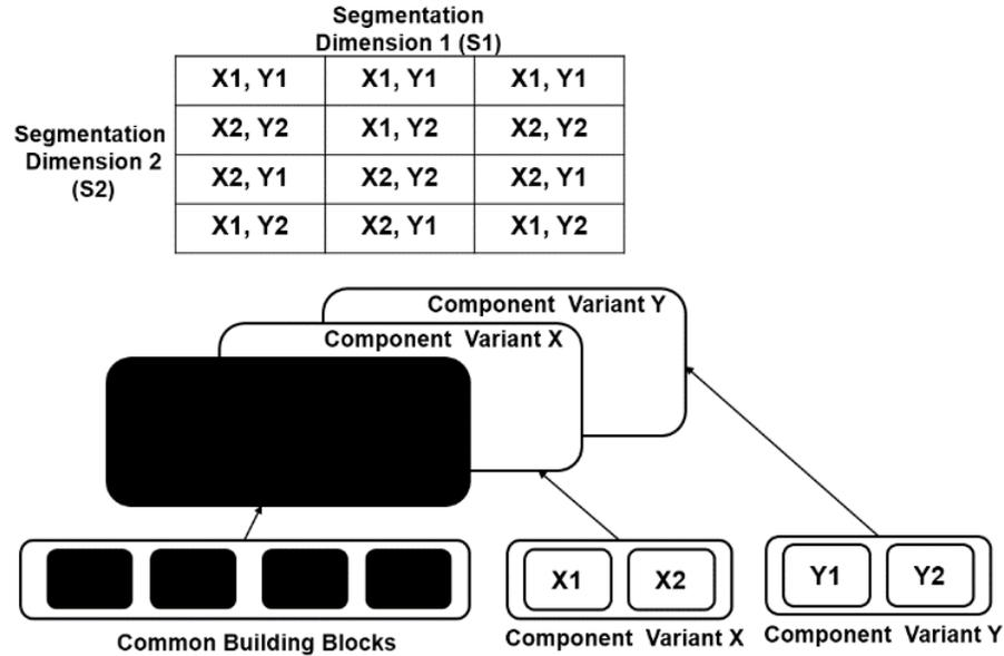
**Figure 1: Redundant variant configurations created from variant choices mapped to market segments.**
