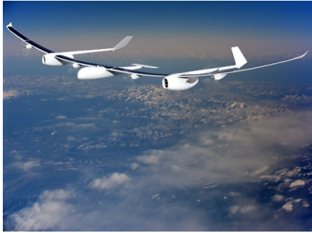
A conceptual study of a high-altitude long endurance (HALE) UAS for a variety of missions such as disaster monitoring, maritime surveillance, and communication relay missions
