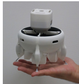
Palm-sized single ducted fan flying robot having high level of safety for harmless to ground objects and people
