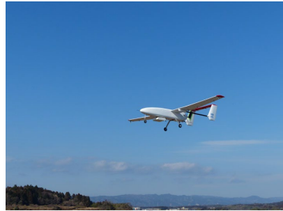
R&D of small Unmanned Aerial Radiation Monitoring System (UARMS) for "Fukushima" in cooperation with the Japan Atomic Energy Agency (JAEA)
