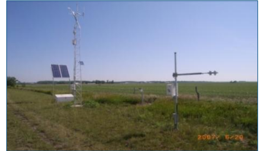
FLUXNET tower, used to acquire time-series environmental data.
