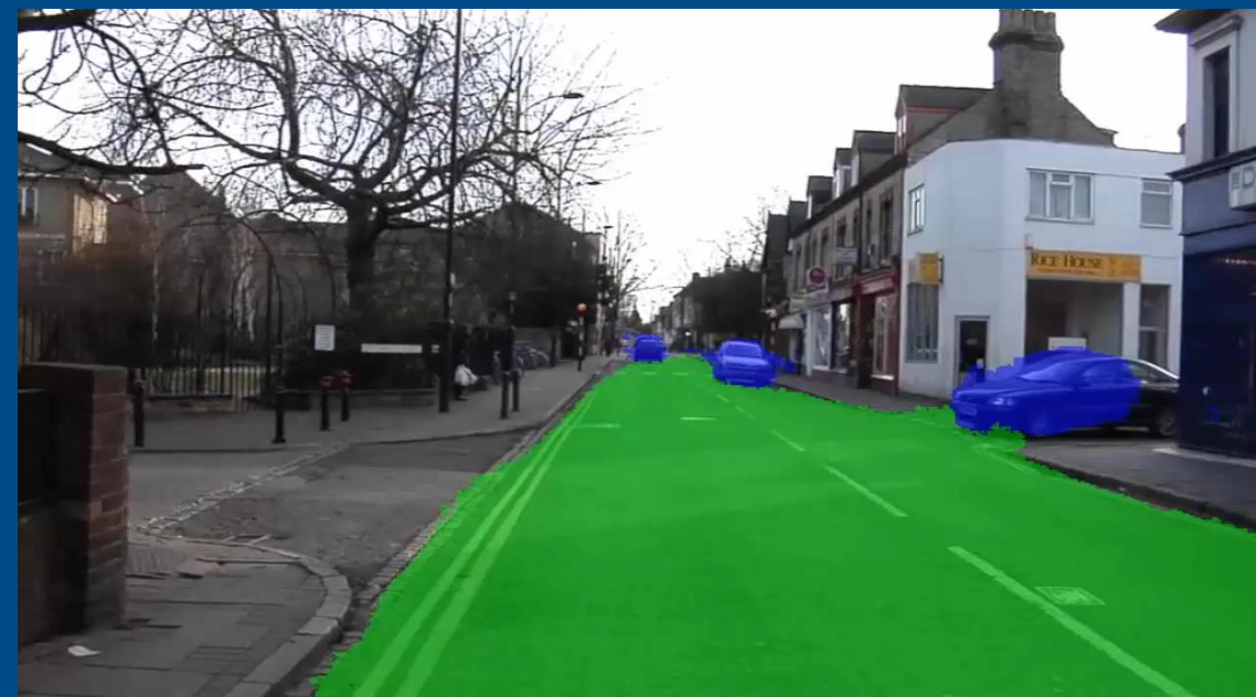
Semantic Segmentation (17b) Automated Driving System Toolbox
